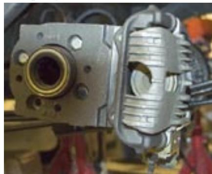
This show how the caliper comes with the standard holes in the bracket. Note how it will interfere with the leafspring. The 4th gens don't have this interference.
