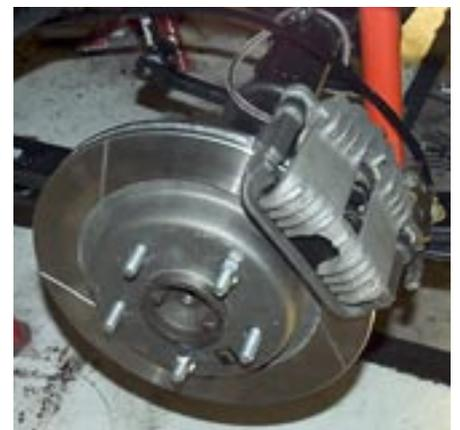
Brackets for the calipers can also be fabricated from steel plates for a sleeker look. If doing so it is very important that the caliper gets centered over the rotor.
